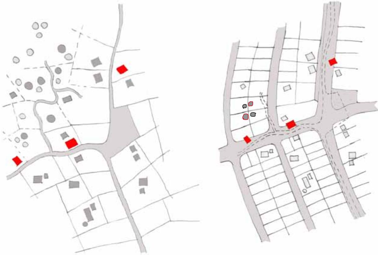
**Example:** regularization of an existing layout with the fewest possible demolitions.
