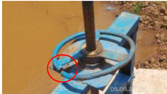
figure 15d: Mechanism to close and open the sluice gate is damaged, it is believed that the rust constantly increases the force needed to open and close the sluice gate, until its breaks.
