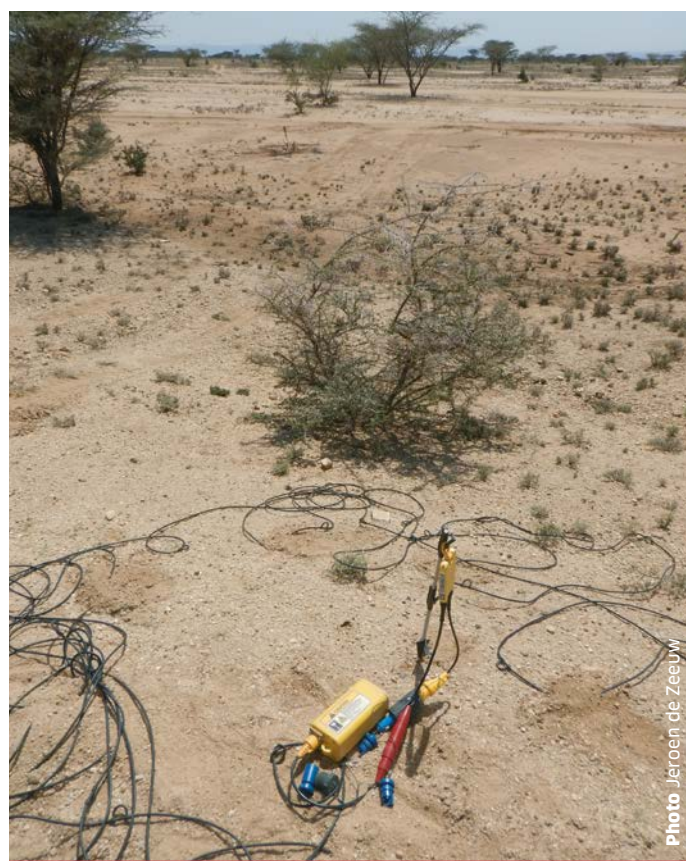
Geophones and cables for seismic surveying.
