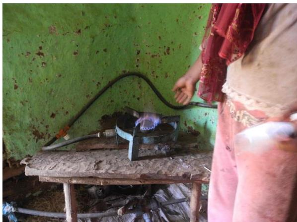
*Photo 27: Stove working with biogas*
